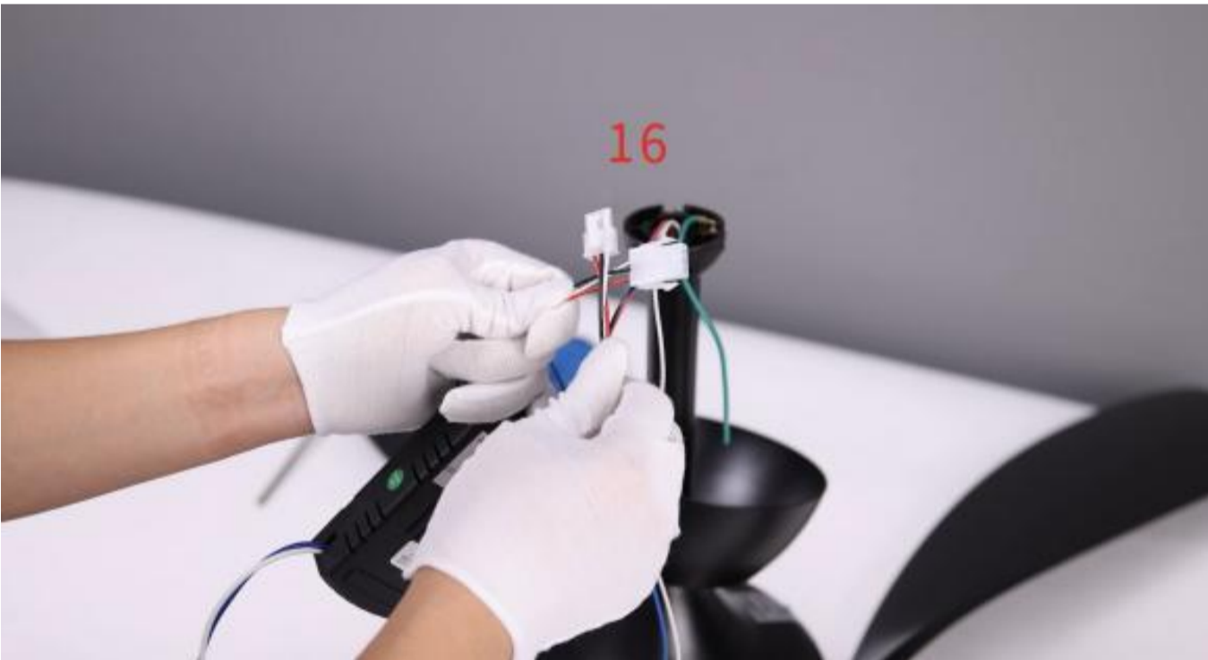
27. Connect the wire from the ceiling fan to the receiver (Red, White and Black wires)
