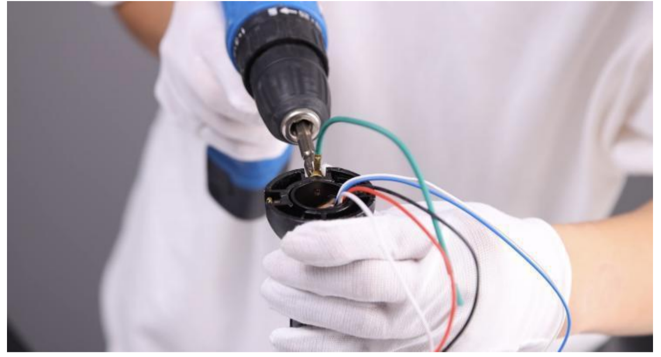
24. Fix the green ground wire with screw. Align the screw hole and tighten the screw
