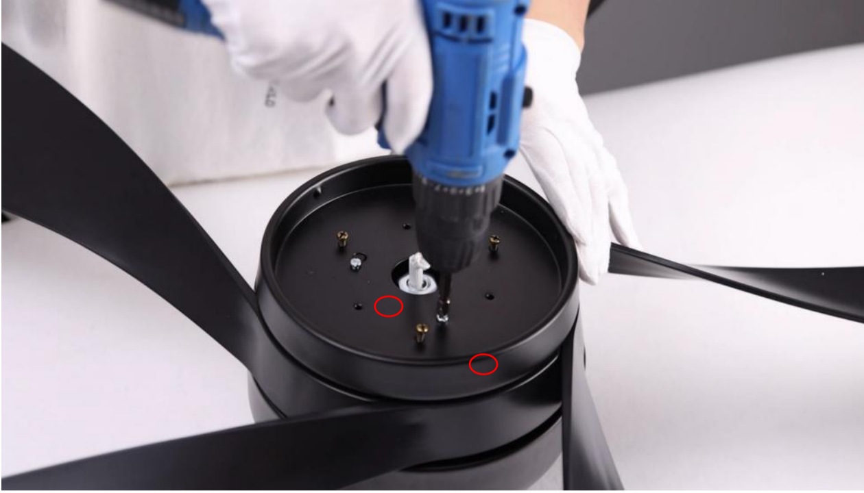
7. Tighten the 3 silver lamp panel screws
