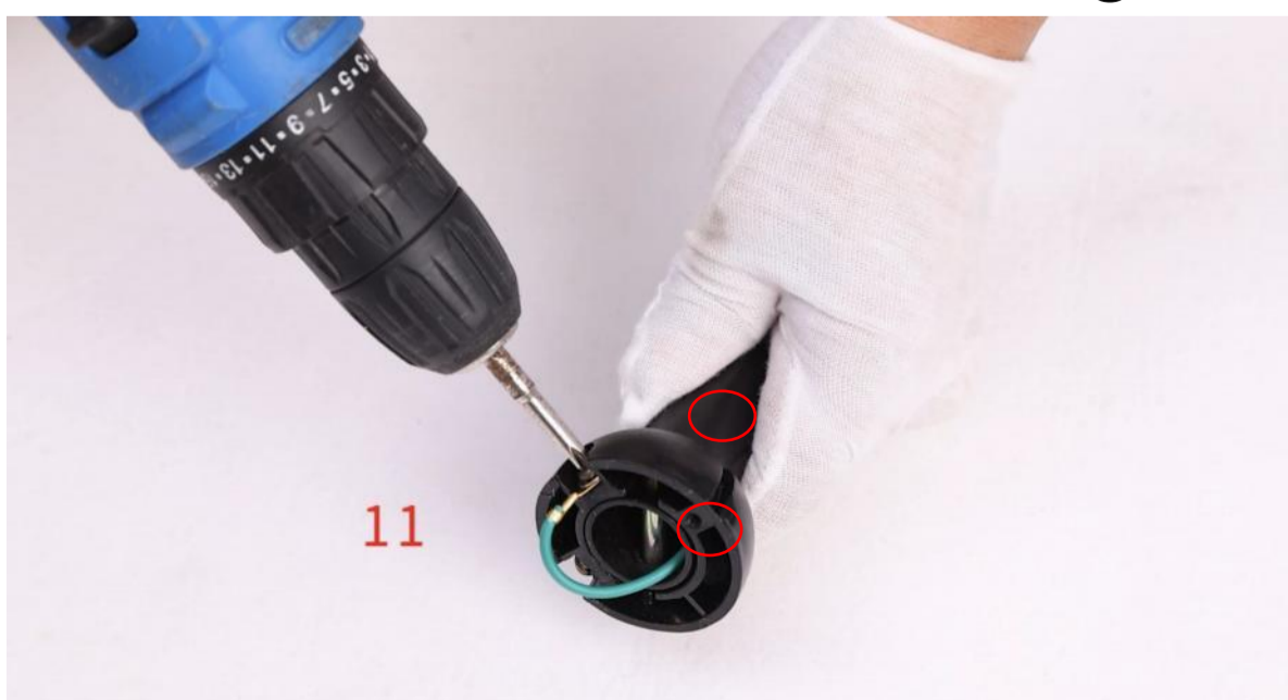
13. Remove 2 screws on the hanger ball
