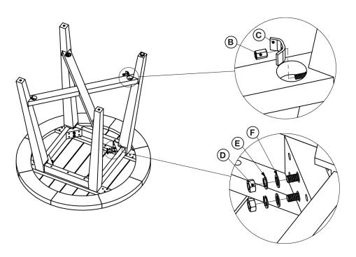
**Step 5** Tighten all bolts completely.
