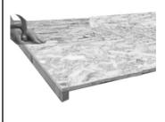
2 Starting from the front place one roof panel flush to the front and sides. Nail into top of framework at front using 8 x 40mm nails and 4 x 40mm nails along each side. Nail into both bearers using 3 x 40mm nails per bearer.
