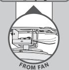
Turn the splices upward and push them carefully back through the hanger bracket into the outlet box. Spread the wires apart, with the grounded wires on one side of the outlet box and the ungrounded wires on the other side of the outlet box.
