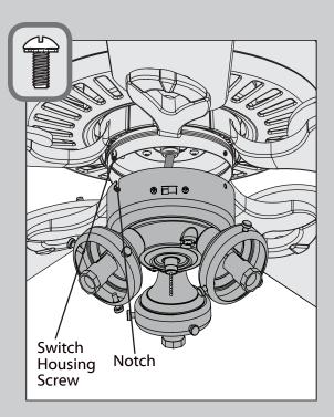
Partially install two of the switch housing screws found in the ≡ hardware bag. Align the notches in the sides of the lower switch housing with the screws on the upper switch housing. Twist the lower switch housing clockwise to lock into place.
