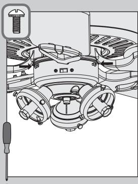
Install the third switch housing screw.
