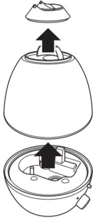
2. Invert the water tank and turn the filter cap counterclockwise.
