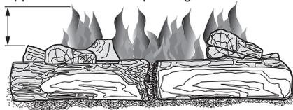
Figure 24 - Correct Burner Flame Pattern
