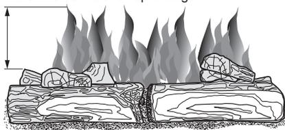
Figure 25 - Incorrect Burner Flame Pattern
