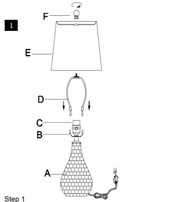
Insert the Harp (D) into the Saddle (B). Put the shade(E) on the Harp(D), then tighten the Finial (F)into the Harp (D)
