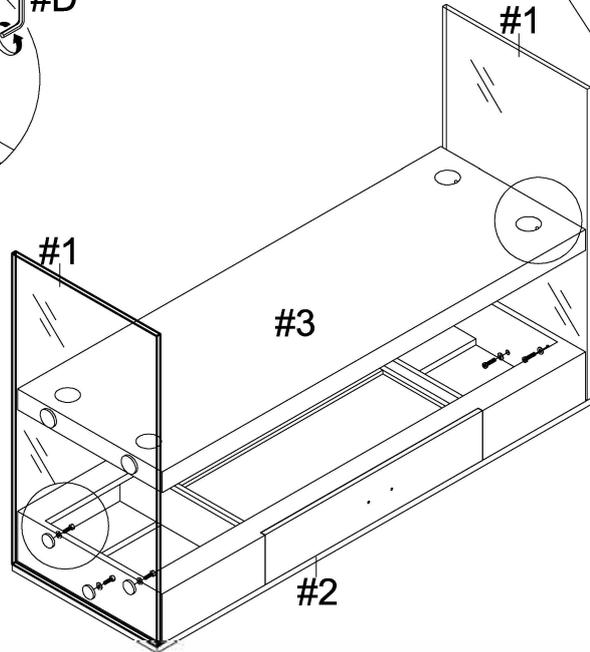
1) Attach rod to the big holes of the side glasses (#1). Insert the rod attached to side glasses (#1) through the holes of bottom shelf (#3). Insert moon washer (#H) to the rod, then secure with hexnut (#C).
