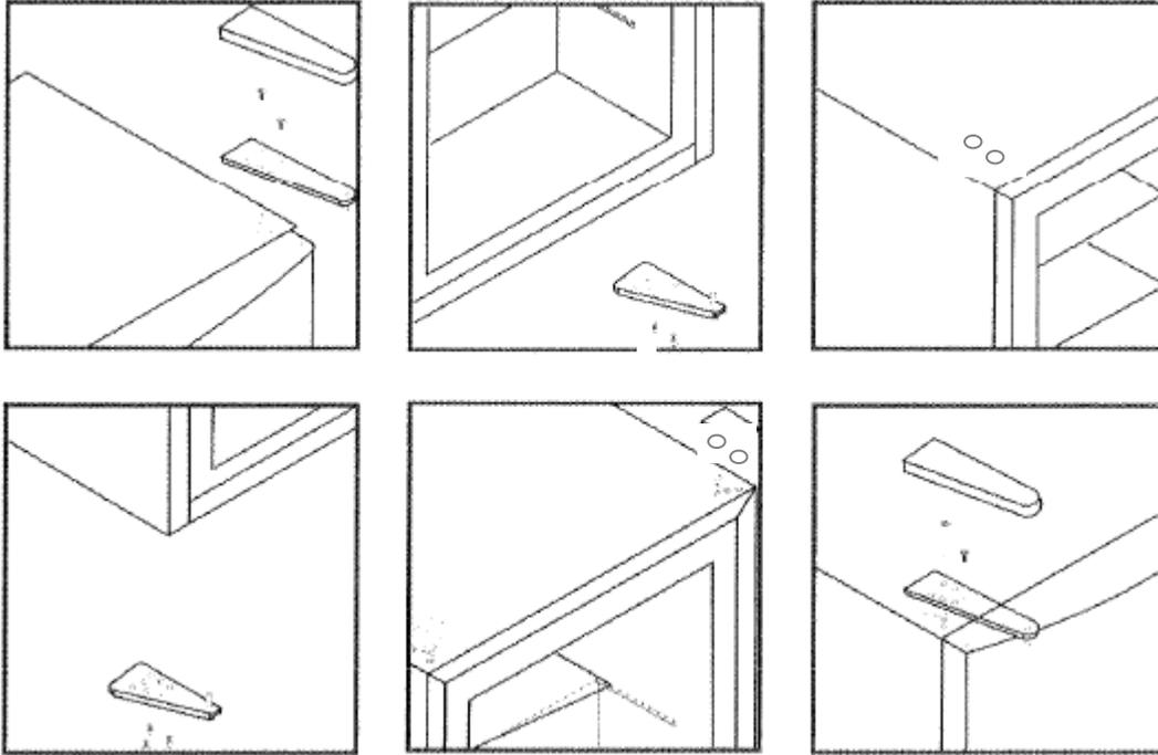
1. Remove the door hinge cover from atop the upper door hinge, and set aside.
