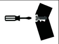
9 Sometimes the laminate might cover partially or entirely the hole on a panel. If there is no visible hole for the screw, pass and press the tip of your finger over the area where the hole should be located to feel the indentation, and once found, carefully pierce the laminate to reveal the hole underneath.
