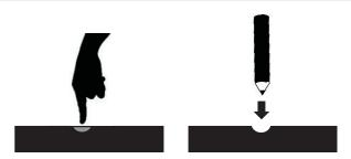
If the hole seems too small for the screw, first make sure you are using the correct size of screw and that it's been installed in the correct hole. If the hole still appears to be too small, carefully pierce the laminate to reveal the hole's actual size.
