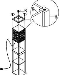
8. Place frame (I) onto short poles (H) and tighten with screw(B).
