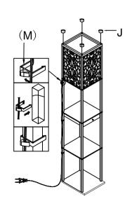
$9.Put\ the\ caps(J)\ onto\ frame(I),\ cover\ the\ screws(B).$  Attach the clamp(M) on the pole to secure the wire , your lamp is ready to use.
