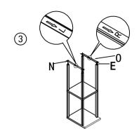
3. Put tracks (N) and (O) into the poles(D), tighten with screw(E) Note: Please make sure the tracks(N) and (O) are placed in the correct direction for drawer(L).
