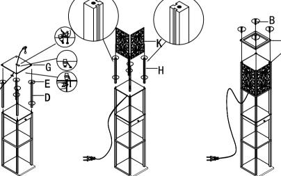
7. Screw the short poles(H) on board(G), tighten to the correct position as above. Slide the shade(K) into short poles(H).
