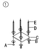
1.Carefully unpack all parts from the packaging and place them on a flat/smooth surface. Be sure to remove all the packaging materials from the lamp. Screw and tighten the long poles (D) to thick board (C) with screws(B), and cover them with cushions(A). Tighten the screw(E) on the top of long pole(D).
