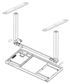
All Parts needed to assemble seen in above figure. Essentially just 4 simple steps of connecting 6 pieces in place.
