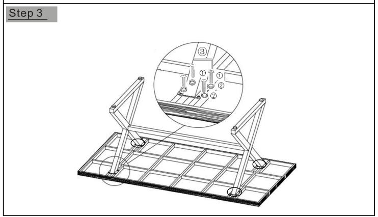
Turn the table top upside down to a soft surface to avoid scratching. Attach Table Leg with Pre-attached Levellers(B) to the mounting position on the table top(A) with Bolts(1), Washers(2) by Allen Wrench(3). **DO NOT OVERTIGHTEN.**
