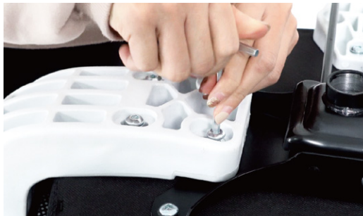
7. Secure the seatback on the seatbase with allen wrench.
