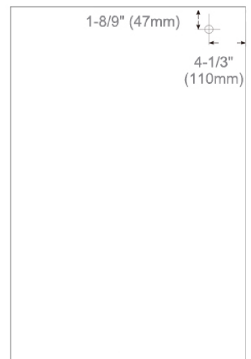
Back of Cabinet - Wire Access Location
