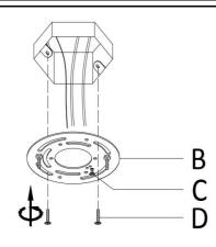
**Step 1:** Unpack all parts from cartons carefully. Separate the Mounting Plate (B) from the Lamp Body (E) by removing the Canopy Nut (F) anti-clockwise. Fix the Mounting Plate(B) to the junction box with Mounting Screw (D).
