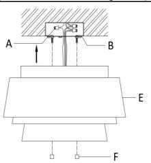
**Step 3:** Attach the Lamp Body (E) to the Mounting Plate (B), and secure with the Canopy Nut (F).
