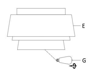
Step 4: Insert the Bulbs (G) into the Socket.
