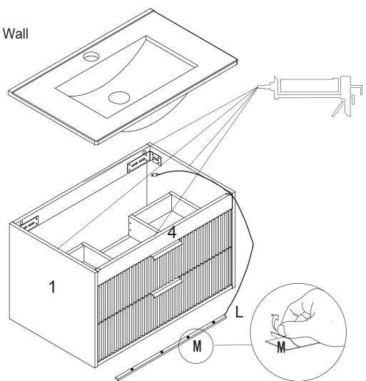
Attention! The wash basin must be bonded to the cabinet using a clear, neutral (solvent-free, neutral curing) siliconebased joint sealant!!
