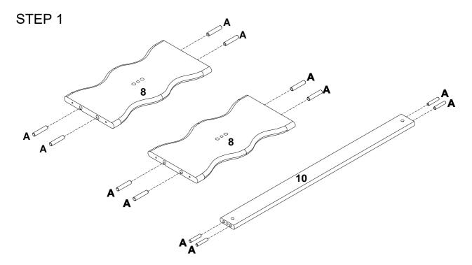
a) Lay Leg Panel (8), Stretcher (10) on a material that does not scratch or damage the parts and insert Wood Dowel (A) into the designated holes as shown.
