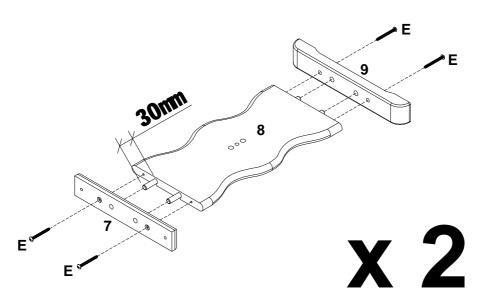
a) Attach Cross-Piece (7) and Leg Base (9) to Leg Panel (8) from STEP 1 via wood dowels on (8).
