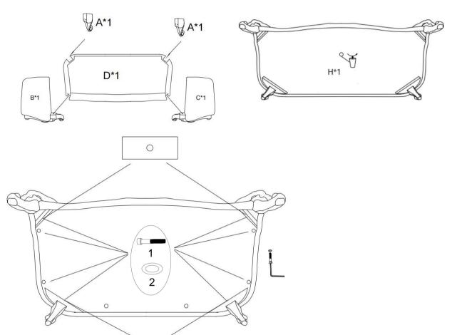
STEP 2 Please hang up the bracket on the backrest into the bracket on the arm.
