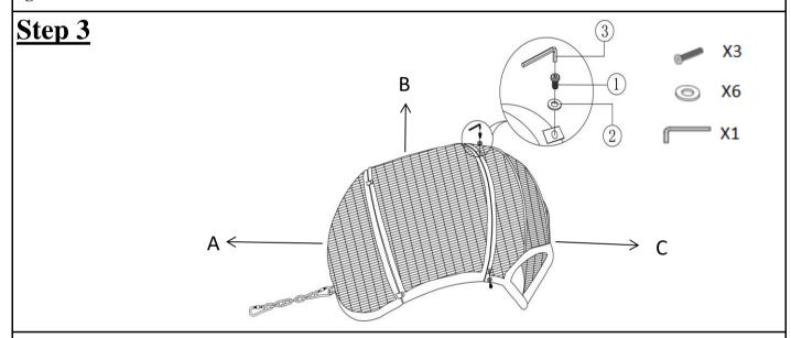
Proceed to assemble Seat (C ) and Back (B) by using Bolt ( 1 )and Washer ( 2 )with Allen Key ( 3 ) . Do not tighten.
