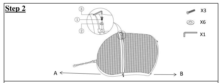
Assemble Top (A) and Back (B) by using Bolt (1) and Washer (2) with Allen Key (3). Do not tighten.
