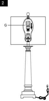
Step2 Insert the Bulb(G) into the Socket(C). Step3 Put the light on a level surface to check if everything is stable.
