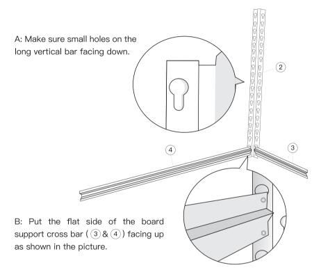
C: Knock on cross bar (3&4) with rubber hammer until the bar covered the small holes completely.
