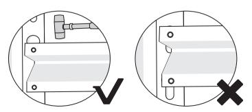
Step 3 Connect another long vertical bar ( 2 ) with the finished part in the previous step by the cross bar ( 4 ).
