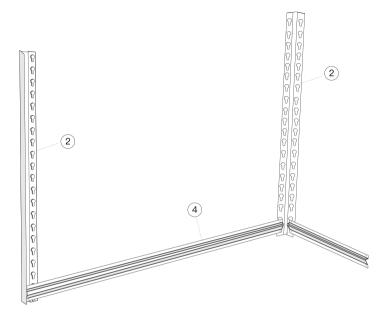
Step 4 Refer to step 2 and step 3, connect the other two vertical bars in turn through the cross bar, as shown in the figure.
