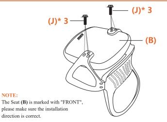
Turn the Seat (B) upside down . Using Wrench (M), install Armrests (C)x1Lx1R to the Seat with Bolts (J)\*6.
