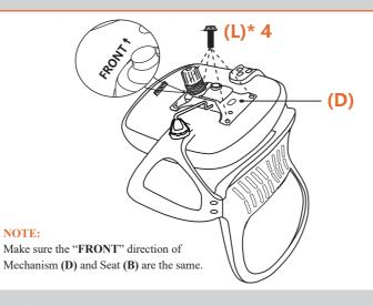
Using Wrench (M), attach Mechanism (D) to the Seat (B) with Bolts (L)\*4.
