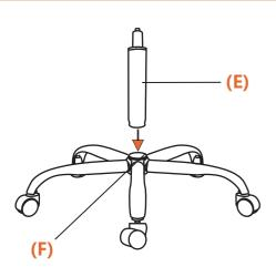
3 Insert the Gas Lift (E) into the Base (F).
