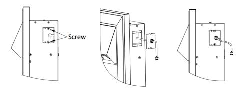
5.4b Carefully mark out the fixing screw positions as below, fit two ST4\*12 screws leaving approximately 4mm between the wall/panel and the screw head.
