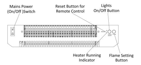
NOTE: The manual button controls basic functions, not a full range of controls. Use the remote hand set to carry out all functions.
