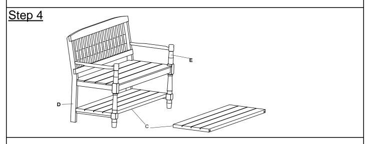
Insert Shelf(C) onto the bottom Rails of Left Leg(D) and Right Leg(E).
