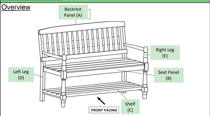
This Bench has multiple parts and may require up to 30 minutes to assemble. To give you an overview of the Bench, the above picture is to help you put the various parts into perspective. Please read through the instructions below to familiarise yourself with the parts and steps before assembly.
