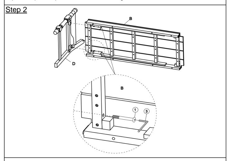
Insert the tenon of the Seat Panel(B) into the mortise of Left Leg(D) and Right Leg(E). Attach Left Leg(D) and Right Leg(E) to Seat Panel(B) using Bolts(1) with Allen Key(3) as shown above.
