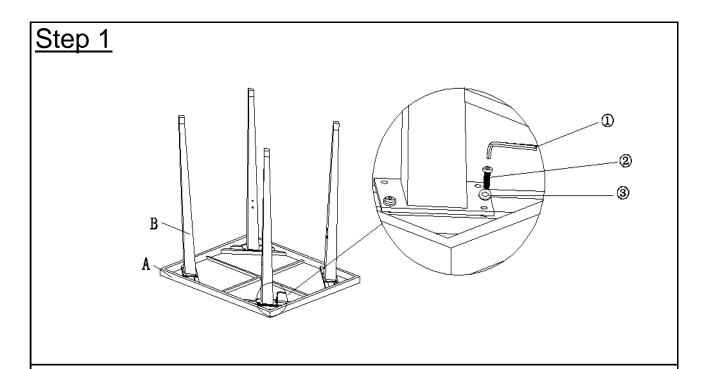
Open the carton and place all the parts onto a clean, non-marring surface. Attach Leg(B) to Table Top(A) using Bolts(②) and Washers(③) with Allen Key(①).
