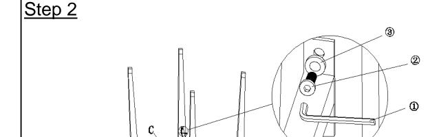
Attach Connector(C) between Legs(B) using Bolts(2) and Washers(3) with Allen Key(1) as pictured.
