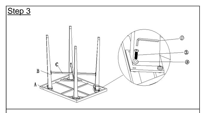
Finally attach Legs(B) to Table Top(A) using Bolts(②) and Washers(③) with Allen Key(①) at the inside mounting positions.
