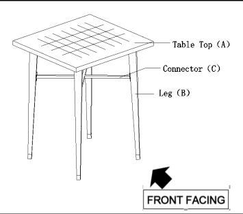
This Table has multiple parts and may require up to 30 minutes to assemble. To give you an overview of the Table parts, the above picture is to help you put the various parts into perspective. Please read through the instructions below to familiarise yourself with the parts and steps before assembly.
