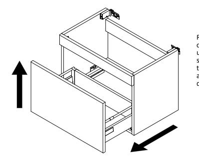
Remove drawer from cabinet prior to fixing unit to the wall. To do so pull-out the drawer to its full extension and gently lift the drawer box upwards.
