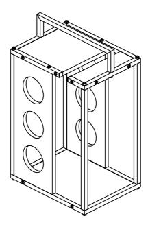
Make sure the unit is rested on a flat surface and does not feel loose or wobbly. If it does, double check all bolts/screws are secured and properly tightened.
