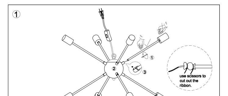
1. Rotate to fix the arms 1 to the ball 2, lock the arms 1 with grub screw.
