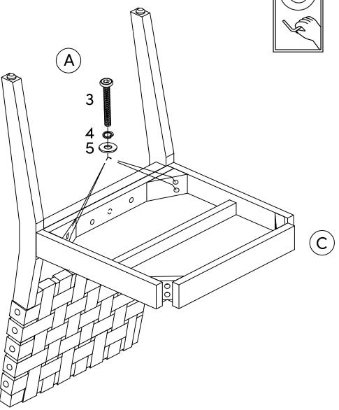
You know what they say, never skip leg day! Attach the Front Legs (D) to the Seat Frame (C) using the Flat Washers (5), Lock Washers (4), and  $\frac{1}{4} \times 2\frac{3}{8}$  inch Hex Button Head Bolts (2).
