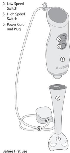
Wash Blending Unit ② in warm soapy water, rinse and dry: the Blending Unit ② is Dishwasher Safe. Beware Sharp Blades in the Blending Unit ② . Wipe the Motor Unit ① with a damp, soapy cloth and dry thoroughly. DO NOT IMMERSE THE MOTOR UNIT ① IN WATER.
