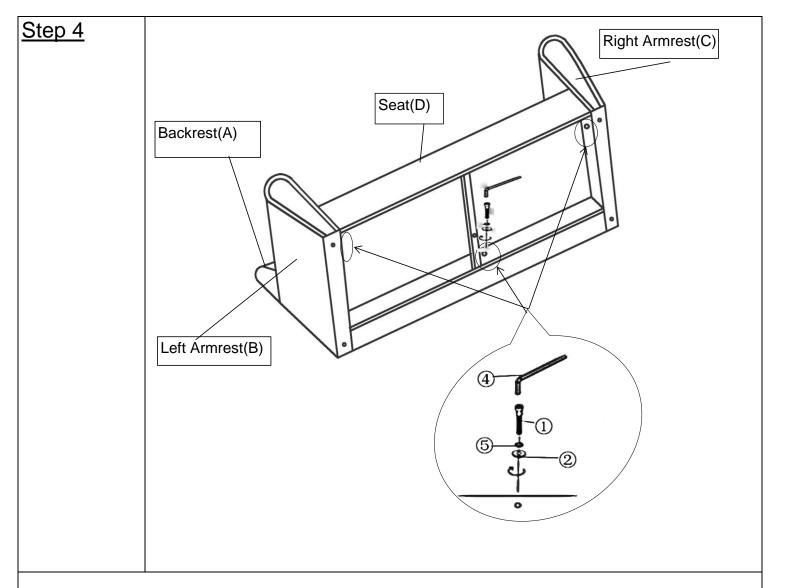
Tilt and lay the Sofa on its Backrest(A) onto a flat surface.
