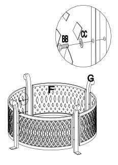
**Step 2:** Attach the Panel (F) with Leg (G) with bolt (BB) and washer (CC). Hand tighten only.
