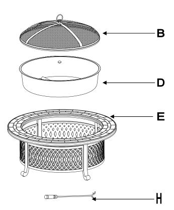
**Step 5:** Turn over the whole assembled piece. Place Fire bowl (D) and Mesh (B) in order.
