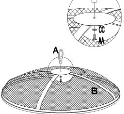
**Step 1:** Attach handle (A) to Mesh (B). Tighten with bolt (AA) and washer (CC).
