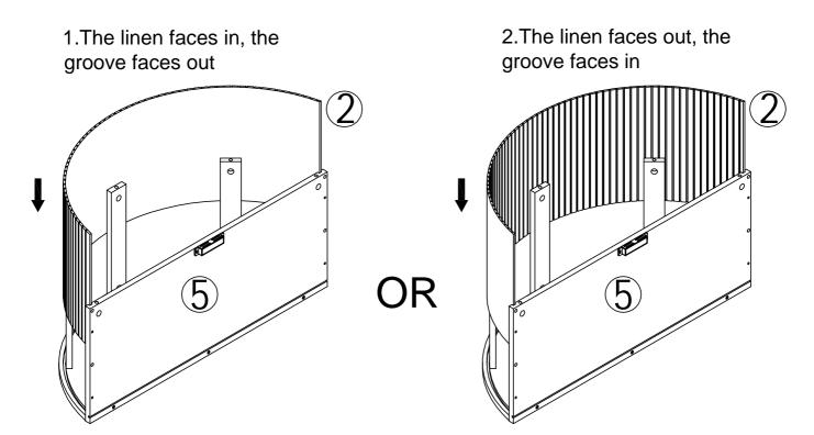
The subsequent installation method is the same. The figure shows only the way the linen faces in and the groove faces out
