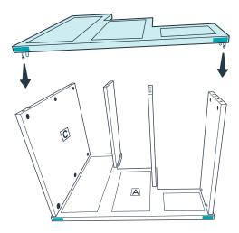
Connect the remaining side panel and secure the connections with cam nuts. Attach the self-adhesive feet to the four bottom corners and turn the steps upright.
