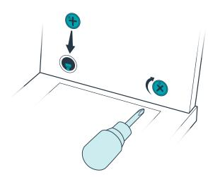
Insert cam nuts into the holes in each riser next to where the panels are connected. (The arrow on the cam nut should point toward the cam bolt.) Tighten the cam nuts to secure the connections.
