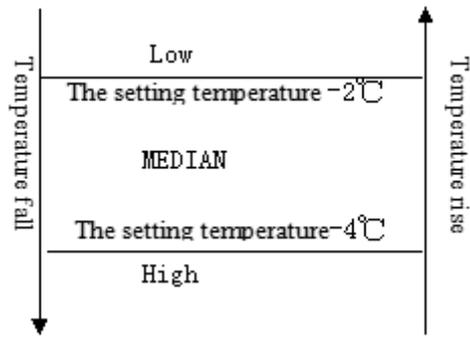
When the difference between the setting temperature and the room temperature equal to 2° or 4° , the indoor fan speed will keep in current speed.
