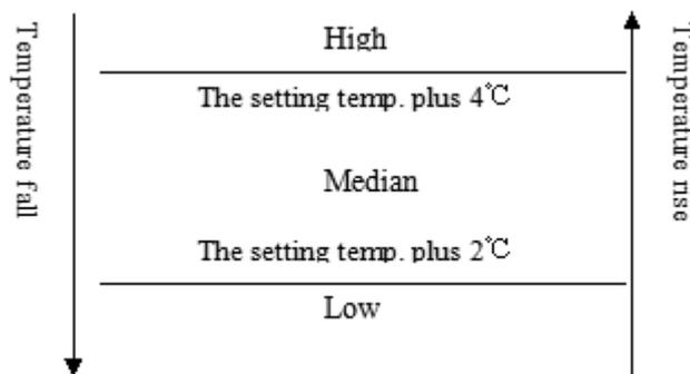
When the difference between the setting temperature and the room temperature equal to 2° or 4° , the indoor fan speed will keep in current speed.
