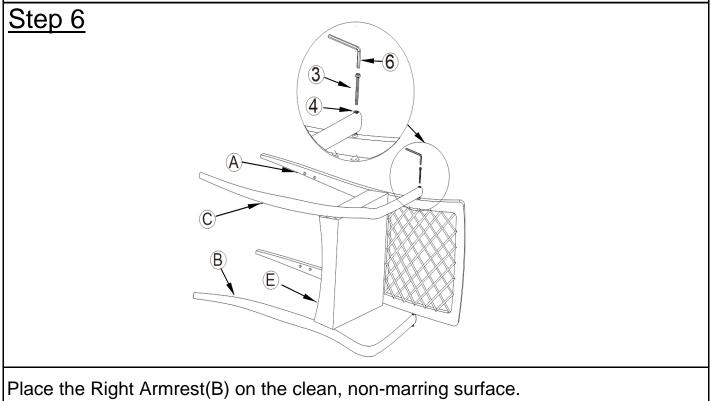
Attach Left Armrest(C) to the Backrest(A) using Bolts(③) and Washers(④) with Allen Key(⑥).
