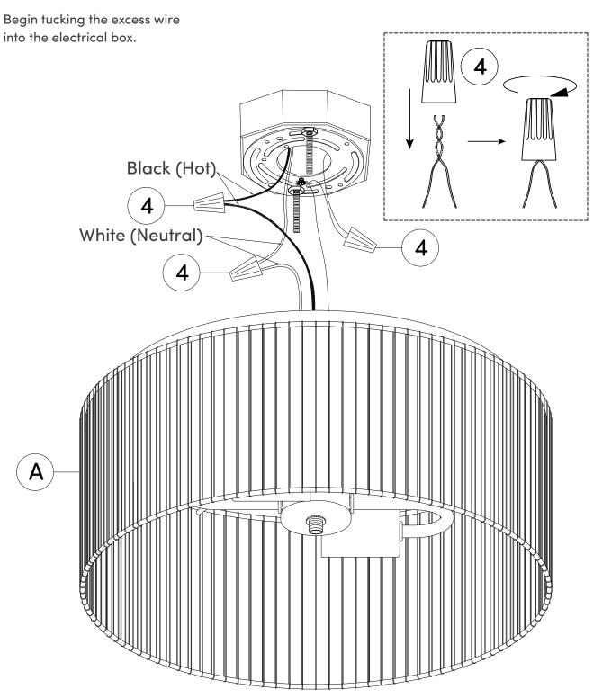
Using the Small Finial Nuts (2), mount the Fixture Assembly (A) to the Mounting Plate (1).
