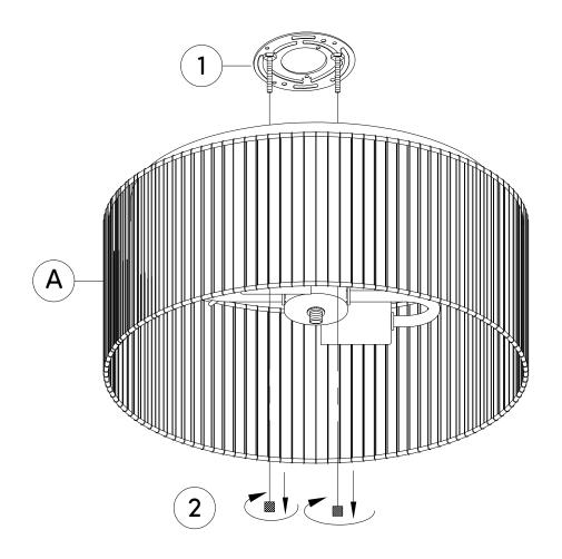
Install the Mounting Plate (1) to your pre-existing Electrical Box, using the Mounting Screws (3).
