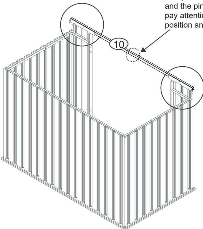
**Note:** The pin hole is on the left door, and the pin hole on 10 should pay attention to the installation position and incline to the left side.
