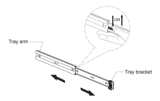
For disassemble drawer tray, by sliding the tray arm and the tray bracket out. Press and tick the small lever on the tray bracket and carefully pull the two piece apart.
