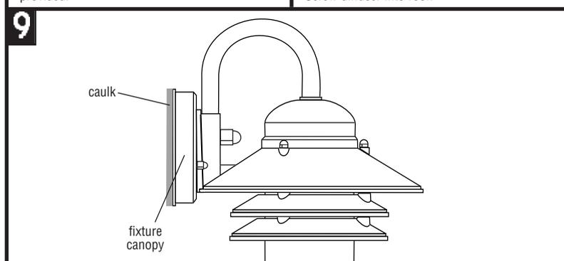
NOTE: Fixture MUST be caulked with an acrylic caulk where fixture meets mounting surface. This provides a water tight seal when fixture is installed.
