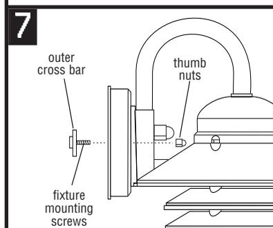
Position the fixture over the fixture mounting screws and secure in place with the thumb nuts provided.
