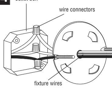
CONNECT THE WIRES. NOTE: Attach black fixture wire to black supply wire, white fixture wire to white supply wire. Do not mix them up. Use wire connectors (not provided).
