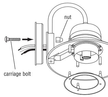
Feed wires from roof thru large round hole in canopy. Align two bosses on canopy with bosses on roof and insert canopy into roof. Be sure canopy fits flush with roof. Insert carriage bolt into square opening in back of canopy, and secure with acorn nut.
