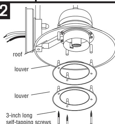
Align posts on top of one louver and insert into holes on bottom of other louver. Align posts on top louver with bosses on roof and secure with 3-inch long self-tapping screw
