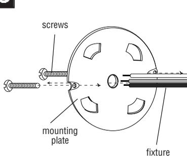
Thread one inch long screws into mounting plate and feed fixture wires through the hole in the center of the mounting plate.
