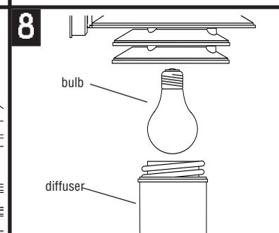
Install bulb into socket. Be sure to use bulb with wattage no greater than specified for this fixture. Screw diffuser into roof.
