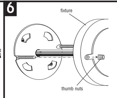
Position fixture over fixture mounting screws and secure with provided thumb nuts.
