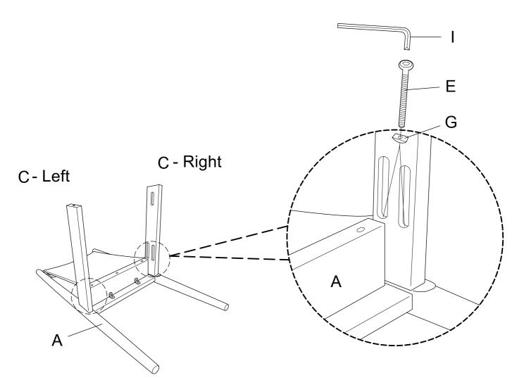
Take the Allen Wrench, and turn the bolts until the legs are secured. DO NOT TIGHTEN COMPLETELY.
