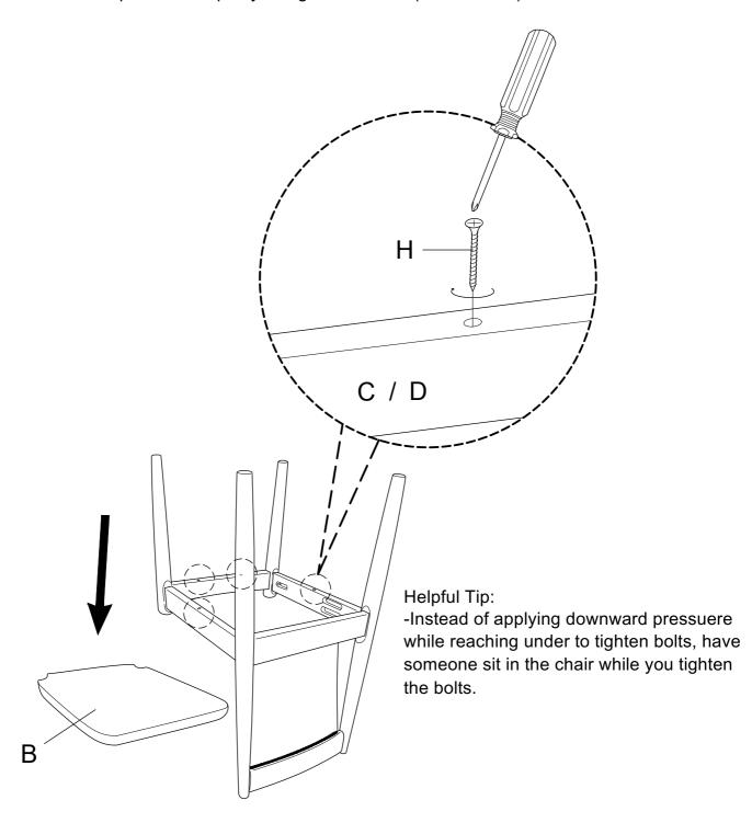
Stand the chair up on even surface and check that it is balanced. If there is a slight wobble, apply downward pressure in the corner where a leg is uneven. Keeping pressure in that corner, tighten all bolts. If balanced, apply downward pressure evenly in the center and tighten all bolts. Do not over-tighten beyond hole depth.
