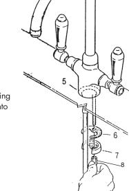
4. Under the sink, stack the half ring rubber gasket - 6, the half ring mounting plate - 7, then the mounting nut - 8 onto the stud.
