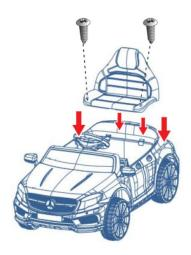
• Put the seat onto the car body according to above picture, and tight the seat with slots well using Ø4\*20 self tapping screw.
