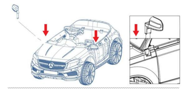
• Make the slots in the mirror in the same line with the slots in car boy and press the mirrors into the gaps.
