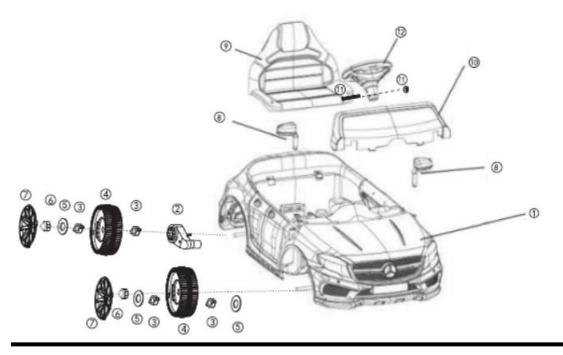
①car body②motors③axle sleeve④wheel ⑤gasket⑥nut⑦wheels cover
