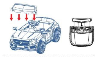
•Check the slot and press the windshield according the slot location to the gap end.
