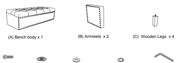
① Bolts x 8 ② Plastic Washers x 4 ③ Flat Washers x 8 ④ Spring Washers x 8 ⑤ Allen Key x 1
