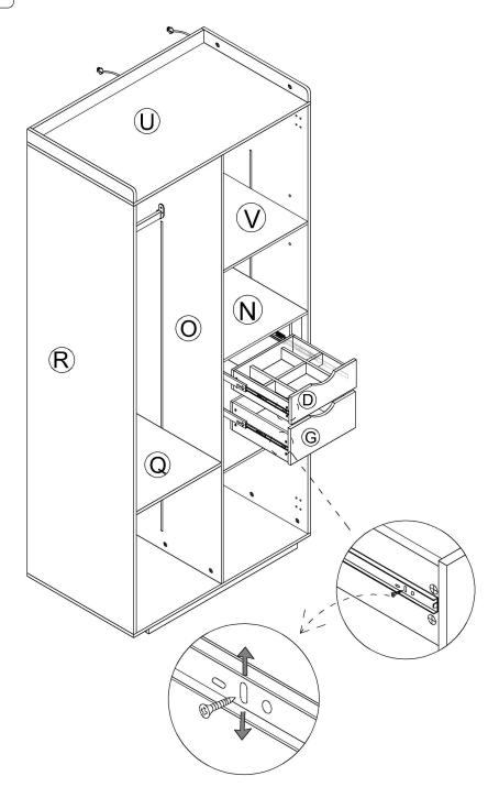
If a large gap is found after installing the drawer the slide rail can be moved up and down to adjust the gap
