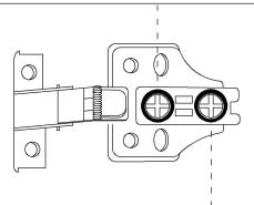
Turn this screw to adjust the door panel to be flat with the side panel.
