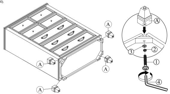
NOTE: MUST TIGHTEN SCREWS PERIODICALLY WITH USE SCREW WILL BECOME LOOSE. CHECK TIGHTNESS OF ALL SCREW EVERY 6-8 WEEKS.
