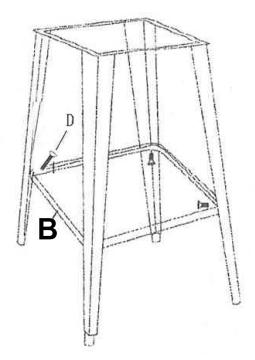
2. Attach Leg Support (B) to each Table Leg (C) using 4 screws (D) .
