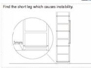
(1).Loosen the screws Loosen the screws between metal frames and bottom 2 wooden boards at the unstable corner and the diagonal corner.
