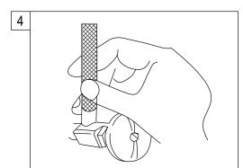
4. Turn on water supply valves and check for leaks, especially at hook-ups to supply lines.
